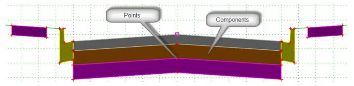
Templates represent cross sectional geometry. A 3D model is created by extruding the template along a 3D geometric path. As the template is extruded the template points connect longitudinally to create 3D surfaces and meshes.
