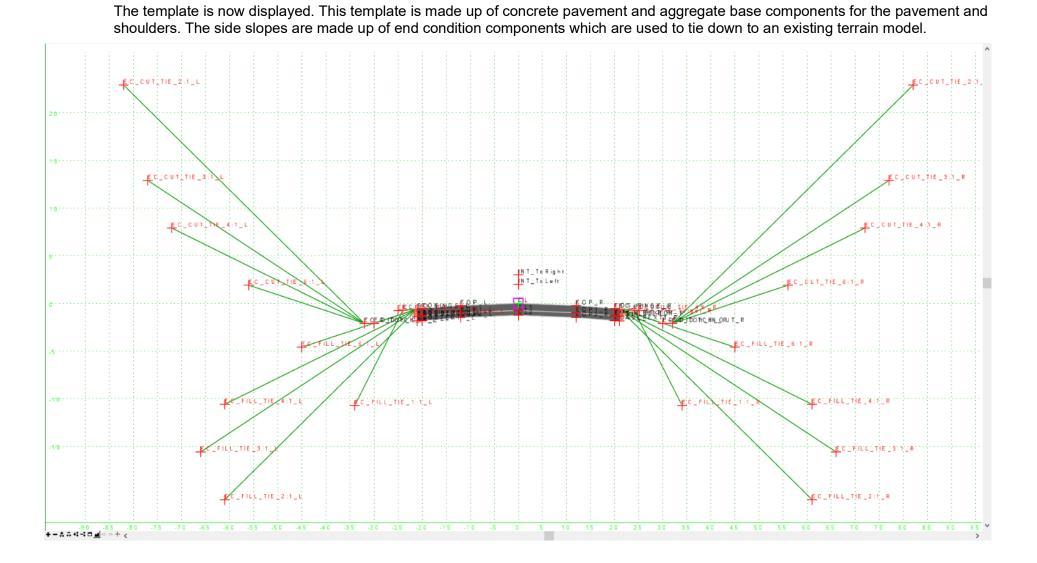
Templates utilize constraints to define the relationship between template points such as the distance or slope between two points. Each point can have up to two constraints which is considered a fully constrained point. A fully constrained points position is fixed relative to its parent point(s). A point with one or zero constraints is free to move in one or more directions.
