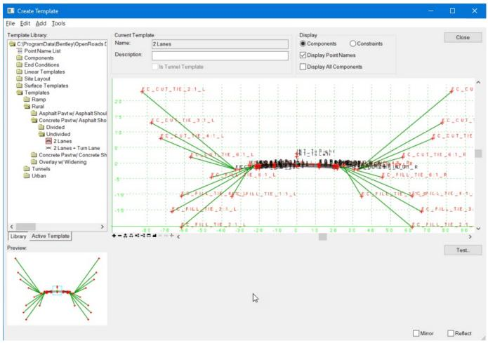
• The templates and components are organized in the template library using a folder structure much like files are stored on your computer. The template folder tree appears on the left side of the dialog.
