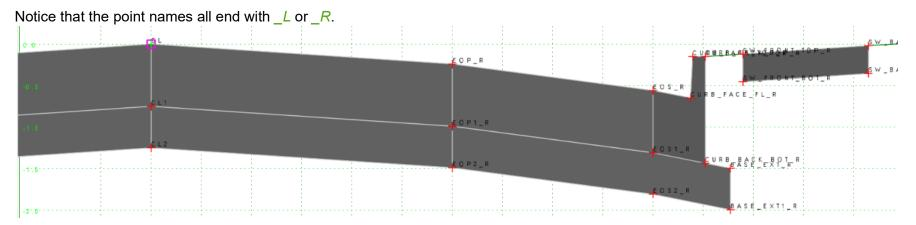
3. Merge common pavement components into a single pavement component.
