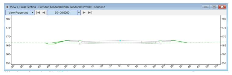
Note that **Dynamic Cross Sections** are displayed in specially defined cross section model views. Any view can be defined to display the dynamic cross sections.
