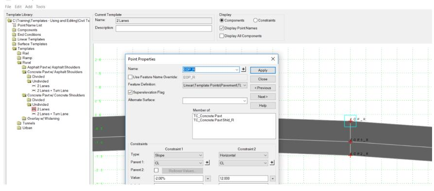
The values in the *Label* fields are know an Parametric Labels or Parametric Constraints. These labels allow the same values to easily be defined across multiple points. In addition, these values can be changed as the template is being extruded resulting in variable thicknesses, slopes, offset distances, etc.
