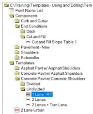
f. Single click on the **1** Lane - RT template and drag it into the template window; while dragging (holding the left-mouse), right-click; When the pop up menu appears release the left mouse button and select Mirror.
