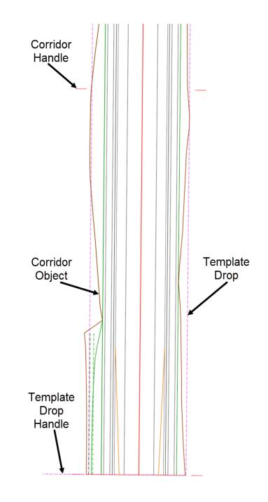
Notice in **View 1**, the closed dashed shape drawn along the corridor. This shape represents the *Template Drop* along the corridor. It has the properties of the template drop assigned to it that you can adjust as needed.
