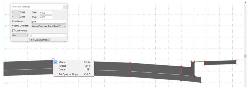
The Mirror option creates a two-sided template from a single sided template. The Reflect option changes its side(s).
