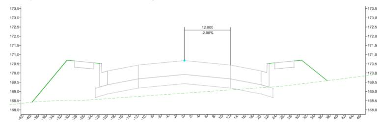
A temporary dimension line will be placed showing the width and slope.
